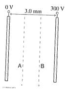
13. What is the electric potential at a point along line A, in between the charged plates?
