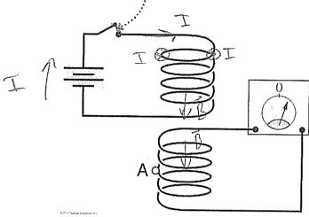
A second coil is connected to an ammeter which measures current in the coil.
